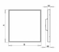
Photometry AERRO III LED - 600 x 600 x 86 mm
