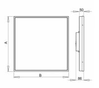
Photometry AERRO III LED - 625 x 625 x 86 mm
