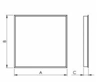
Photometry ARRC LED SQ - 620 x 620 x 70 mm
