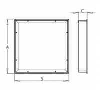
Photometry FOGGY IP65 T5 - SQUARE - 620 x 620 x 97 mm
