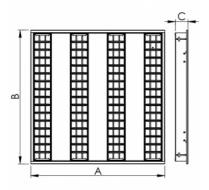
Photometry VARRIO T5 - TRIO-POOLED - 595 x 595 x 57.5 mm
