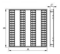
Photometry VARRIO T5 - TRIO-POOLED - 620 x 620 x 57.5 mm
