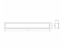
Photometry CANNES T5 - 895 x 105 x 91 mm
