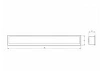
Photometry CANNES T5 - 1495 x 145 x 91 mm
