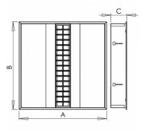
Photometry ROOF - 595 x 595 x 111 mm
